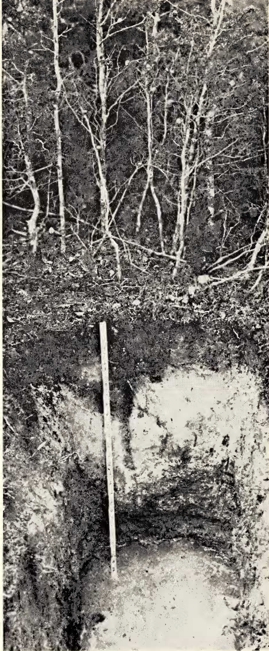
FIG. 2. Pygmy forest—podsol ecosystem. Cane-like Cupressus pygmaea growing on Blacklock soil showing surface humus horizon on white bleached A2 horizon which rests on iron hardpan. Water table is at 66 cm depth. Photo R. A. Gardner.
